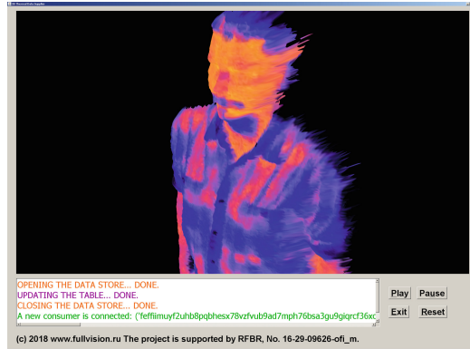
Fig. 1. An example of a logical agent that collects and transfers heterogeneous multi-channel data (3D video data and thermal imaging data).
